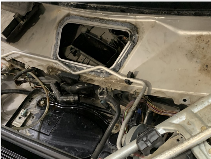
Above: Foam (left) from the blend door (right) Below, heater core access
