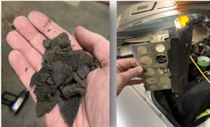
Above: Foam (left) from the blend door (right) Below, heater core access
