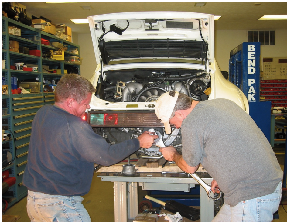
Bob Lynch shared this photo of Sandy Steckman and Jim Avila installing a harmonic pulley on a 964. It needed to be torqued to 174 ft. lbs. You'll want to see this photo on the GPR web page to see Sandy's red face and Jim's muscles.
