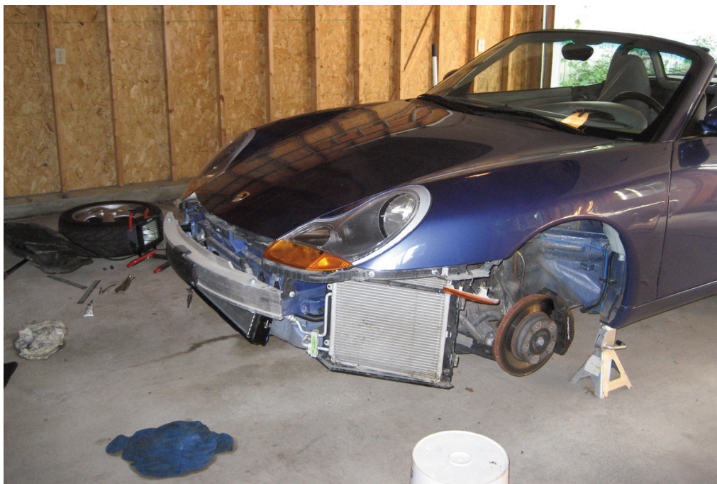
Steve Wilwerding's conversion to the 996 engine required adding a central radiator, visible below the bumper.
